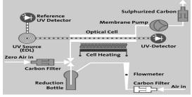
Figure 1. Schematic flow diagram of mercury analyzer
